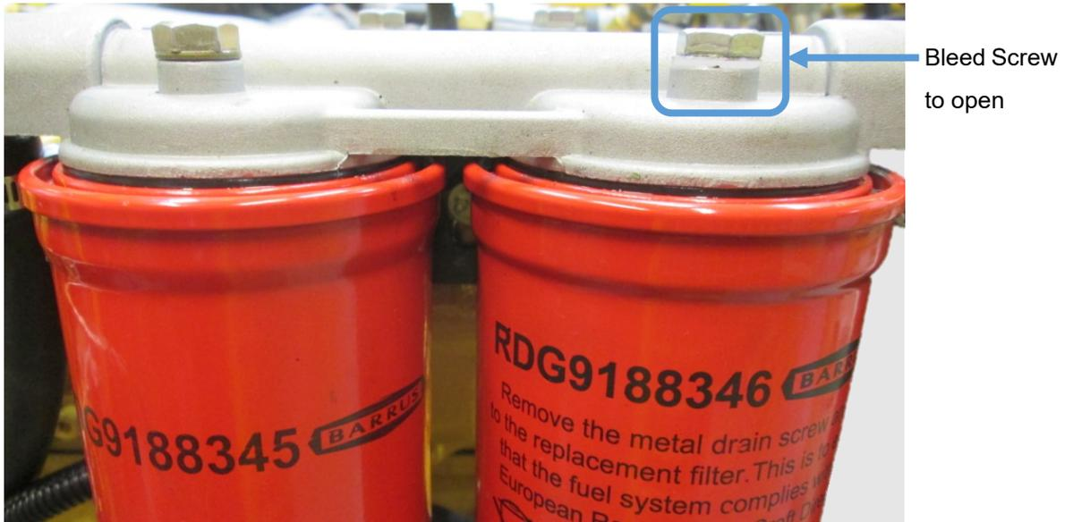
Figure 24: Fuel Filter Bleed Screw
