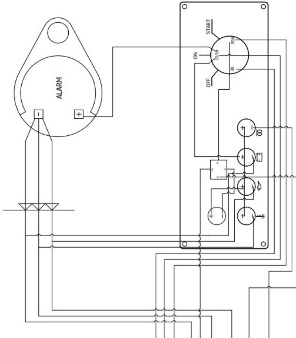
Figure 27: Basic Control Panel Wiring Diagram (Twin Alternator Engines)
