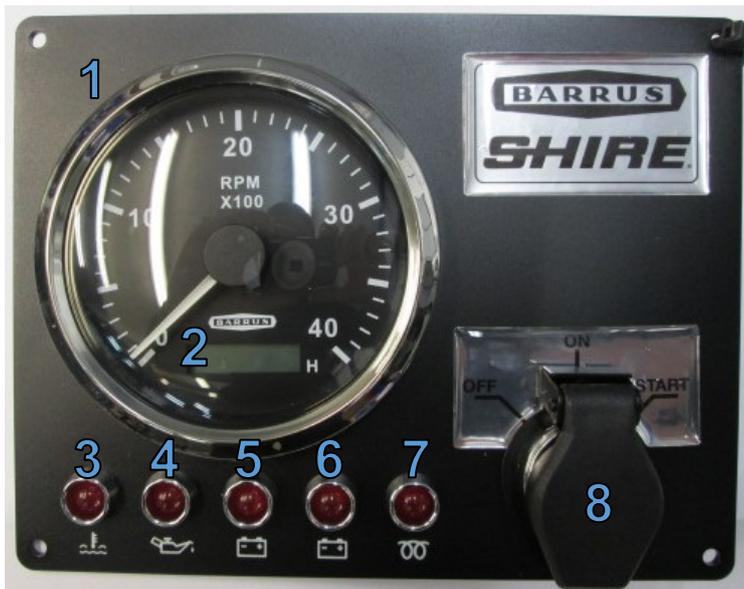
Figure 9: Standard Control Panel
