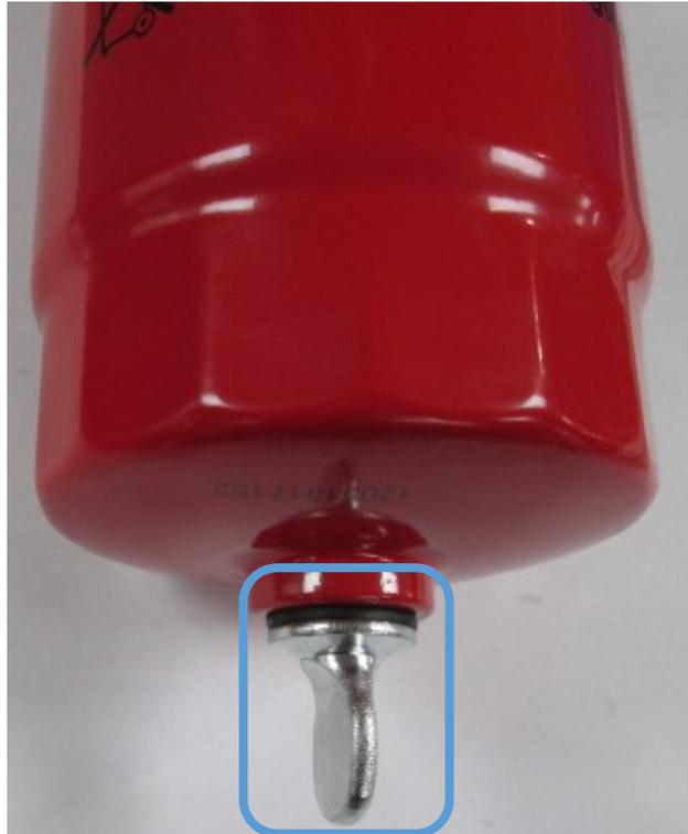
Figure 23: Primary Fuel Filter Drain Screw
