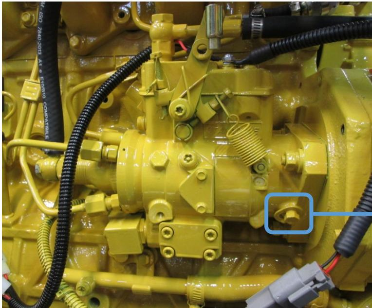
Lock pin in the unlocked position
