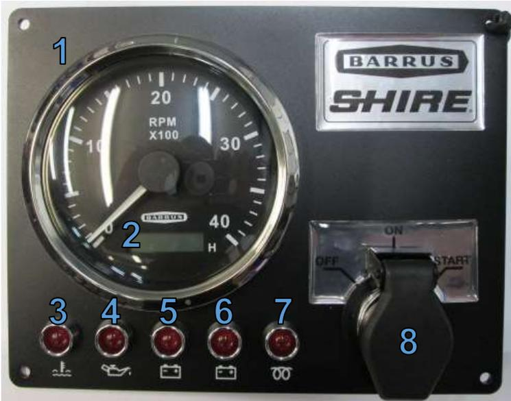
Figure 6: Standard Control Panel
