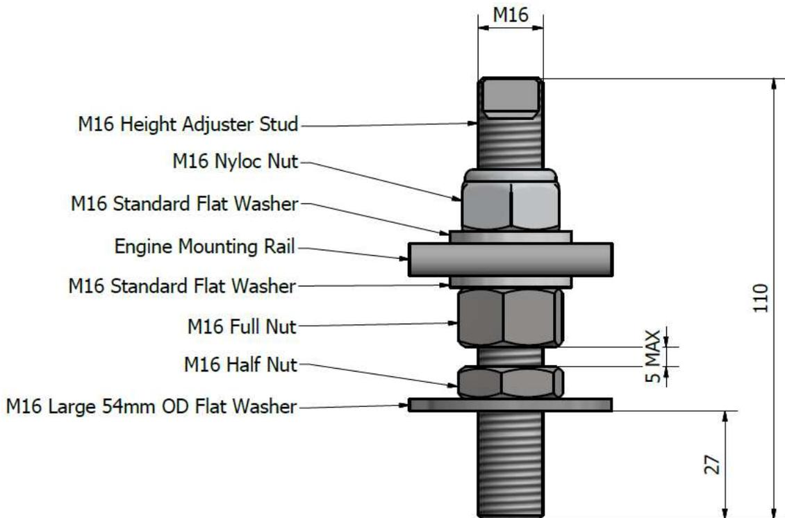
**Figure 13: Correct Anti-Vibration Mount Installation**
