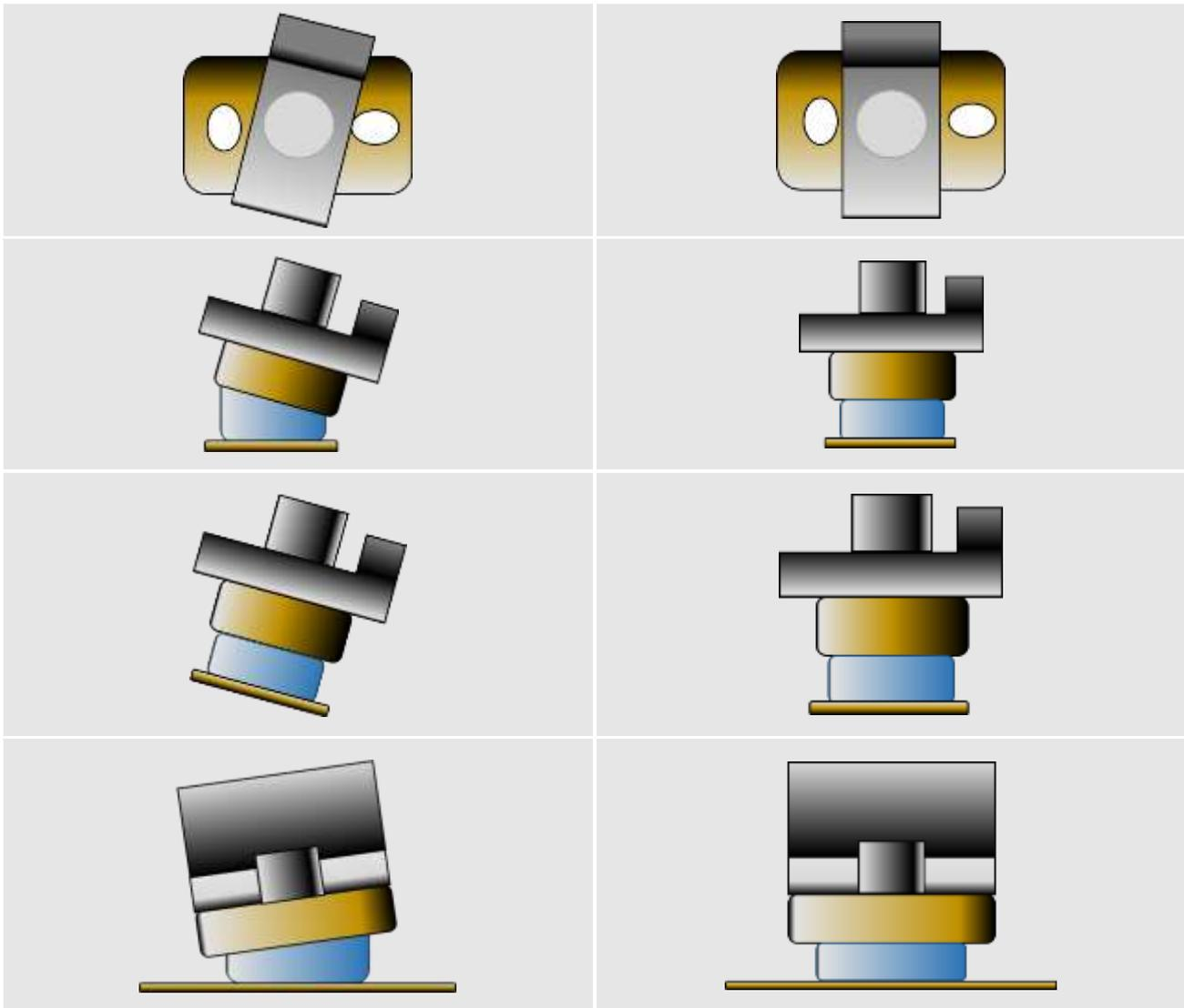
Figure 12: Correct Anti-Vibration Mount Installation
