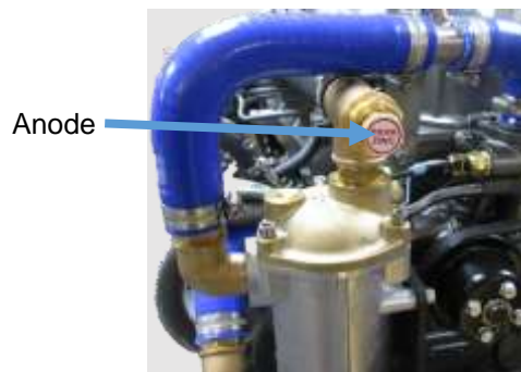
Figure 19: Work Boat Anode Location
