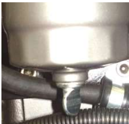
Figure 18: Primary Fuel Filter Drain Screw
